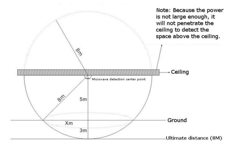
As shown, the actual detected horizontal distance can be calculated.
